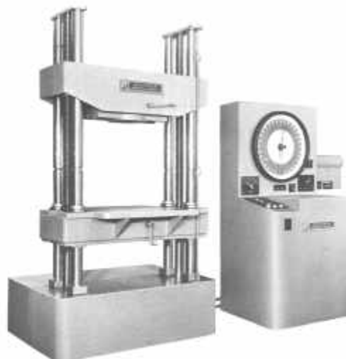
▲ Baldwin's model CS featured a single test space
