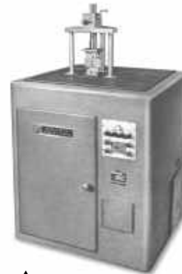
▲ Sonntag fatigue machine with tension/ compression fixtures
