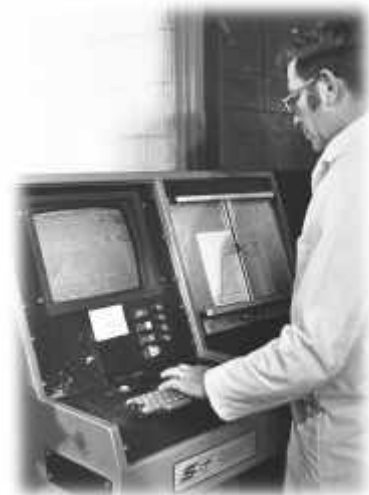
▲ The MATS I controller made possible computer controlled testing
