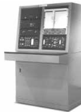
▲ Control console with Mark II digital indicator
