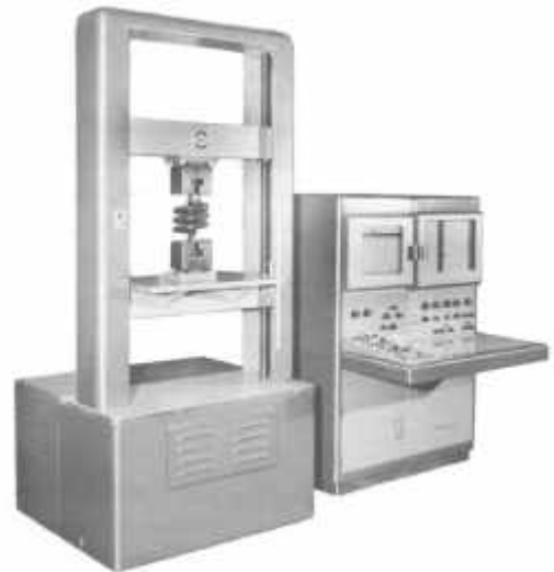
▲ Mark G Series featured a combination servohydraulic/ electromechanical design
