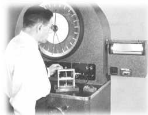
▲ Load versus deformation graphs were made possible with the addition of XY recorders (right of dial)
