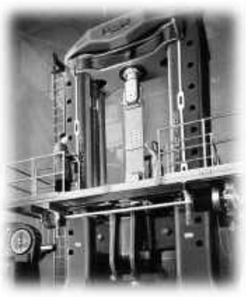
▲ 3,000,000 lbf Southwark-Tate-Emery universal testing machine with tensile specimen loaded
