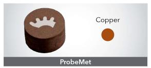
A copper and mineral filled phenolic thermoset recommended for SEM analysis of specimens when copper is not the object of analysis. Note: Can cause a Cu-Al galvanic couple on Aluminum specimen.
