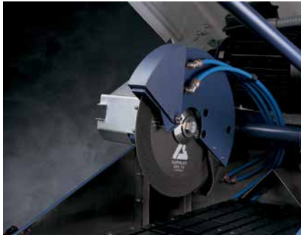
Wheel guard pivots open for easy wheel changing.
