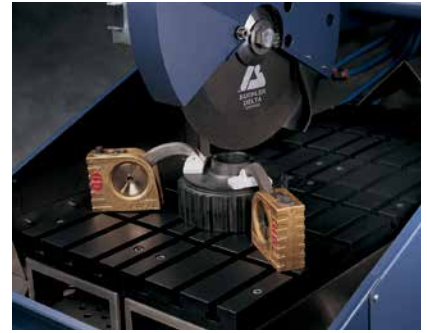
10-3523 Irregular Specimen vises secure unusual sample sizes.
