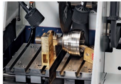
Speed vise and riser blocks provide vertical clamping forces for large and irregularly shaped samples.
