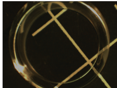
Figure 15.2. Quartz tube after 6 \mu m polish.
