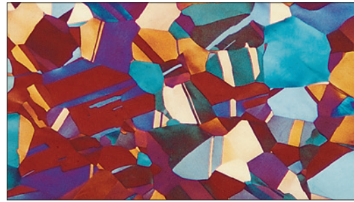
Figure 10.1. Alpha grains containing annealing twins in phosphorous-deoxidized arsenical bronze that was annealed and lightly cold drawn (Klemm's I reagent, polarized light, 50X).
