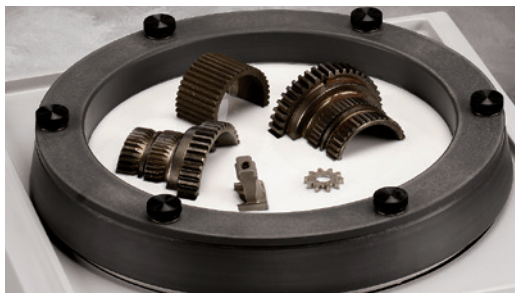
Figure 3.19. Sample preparation with their own weight.
