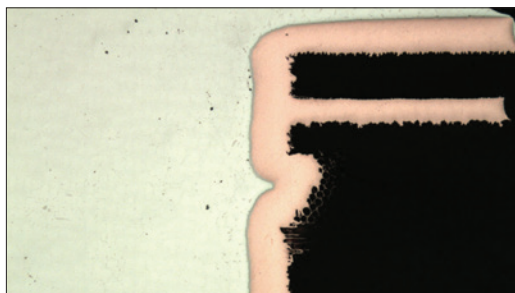
Figure 18.3. Pb-Free Solder in Plated Through Hole, 200x.
