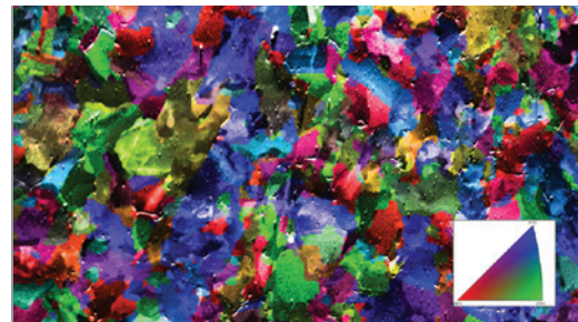
Figure 3.18. Vibratory polished ferritic steel, Electron image overlaid with orientation map normal direction Phase: \alpha - Iron.
