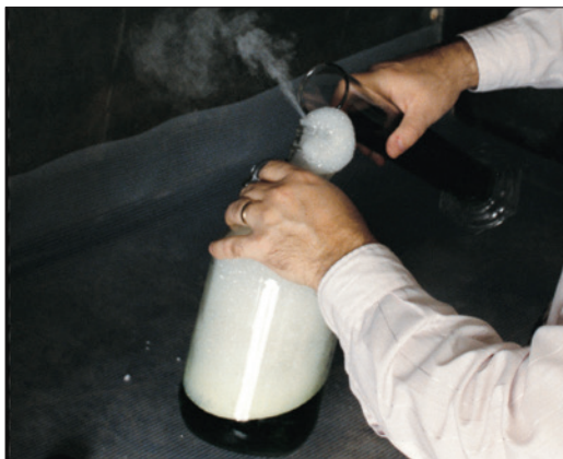
Figure 24.3. Illustration of a bad mixing practice. The acid ingredient was poured into an empty acid bottle and the solvents were added without stirring or cooling. The solution may erupt in the metallo-grapher's face at any moment. It is recommended to keep the hands clear of the area and remove rings.
