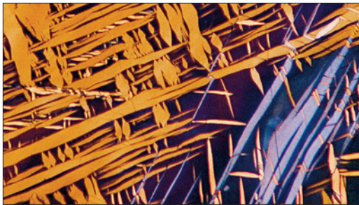
Figure 6.3. Mechanical twinning in deformed high-purity magnesium (99.8% Mg) (acetic-picral etch, crossed polarized light plus sensitive tint, 50X).
