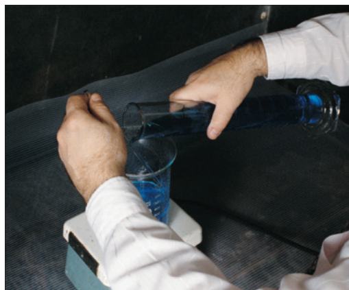
Figure 24.2. When mixing etchants, use a magnetic stirring plate with a magnetic bar for stirring. Slowly add the liquid ingredients to the solvent by dripping them down a glass stirring rod. If the solution is more dangerous than this one, wear protective gloves and use a face shield. If mixing generates substantial heat, it is a good practice to place a cooling jacket around the beaker.
