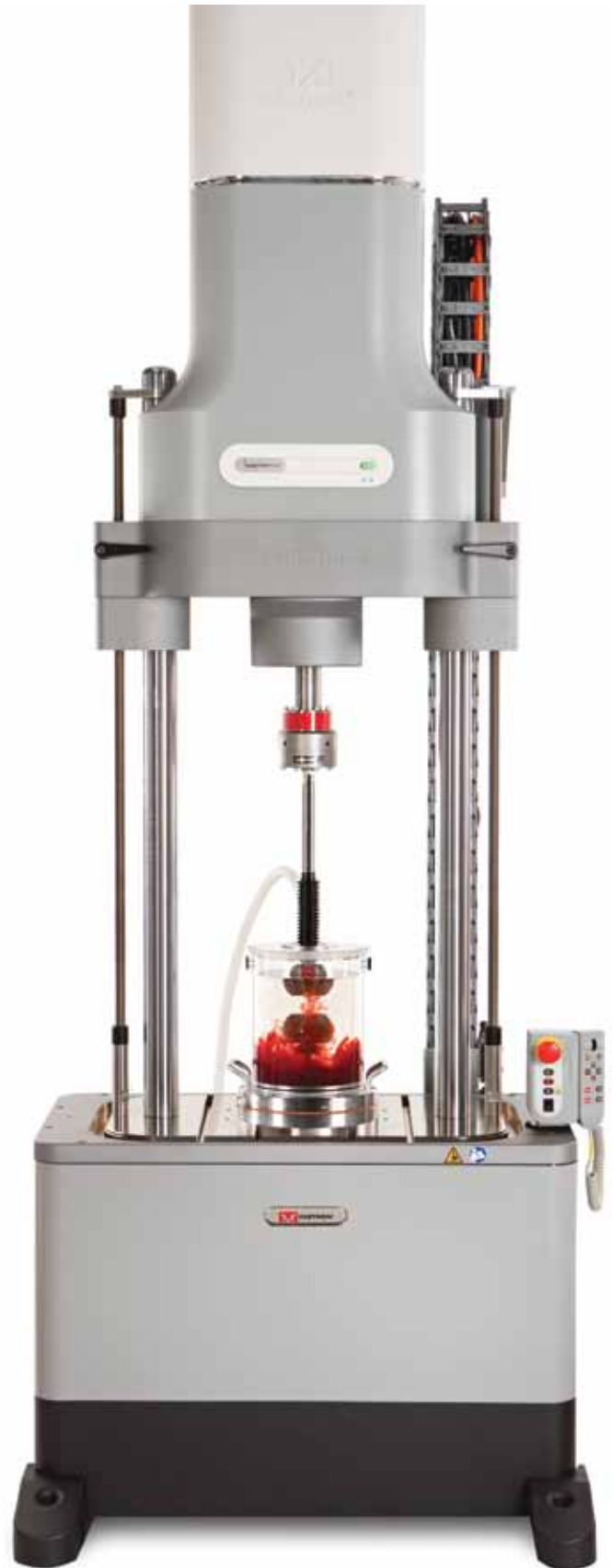
The ElectroPuls™ E10000 Linear-Torsion test instrument can be fitted with a saline bath for long-term fatigue tests, or can be used to perform combined linear-torsion tests on whole bones.
