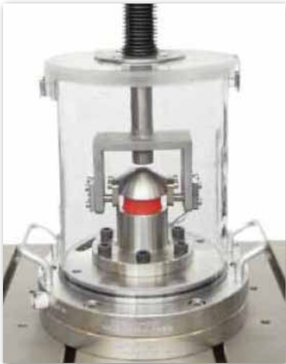
Intervertebral body fusion devices can be tested to ASTM F2077 and F2267 on either the ElectroPuls™ or 8870 servohydraulic fatigue systems.
