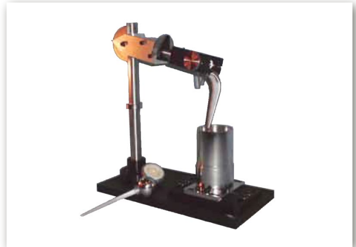
The embedding fixture ensures correct implant alignment for the test
