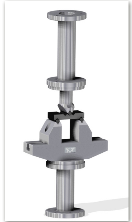
Pullrod with 3-Point Bend Fixture
