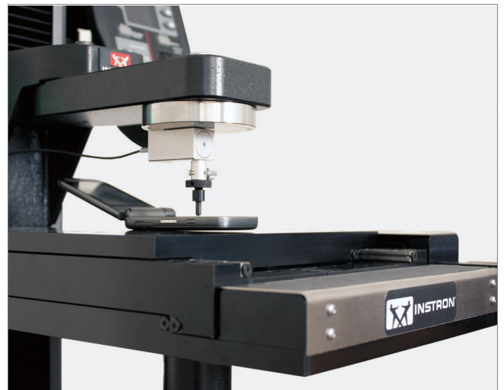
Facility Testing on Multiple Cell Phone Buttons
