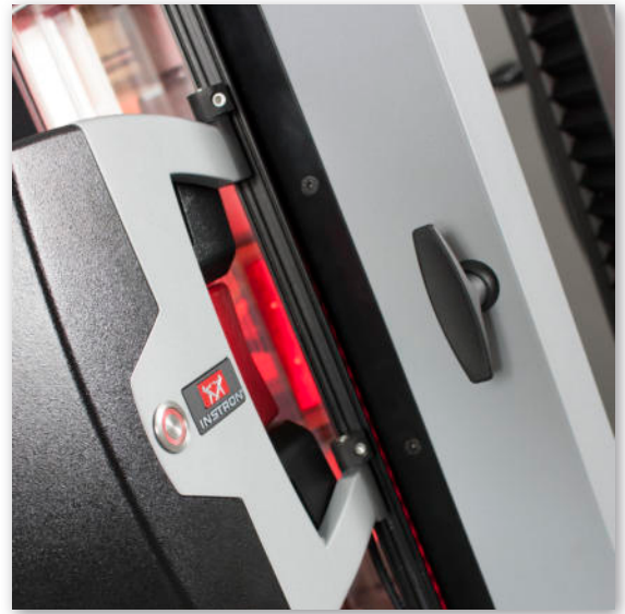
AVE 2 Mounted on a Temperature Chamber
