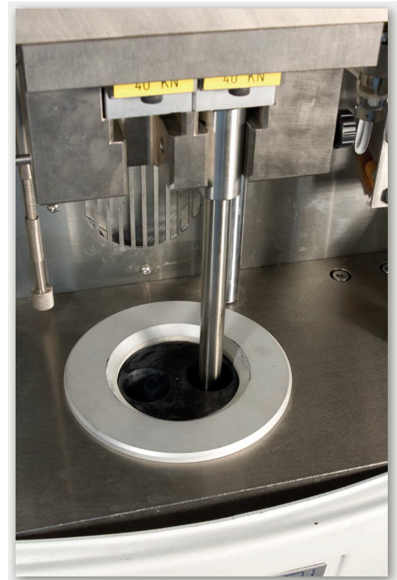
Twin Barrel configuration with two independent Load Cells
