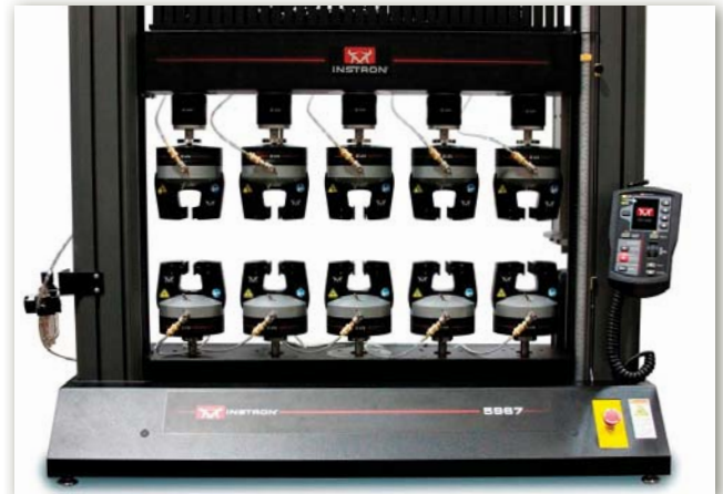
Typical Multi Station System
