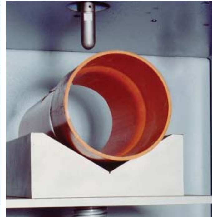
V-Block Support Fixture for Pipe Testing
