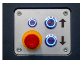
Automatic and manual stage movement are available on the Wilson UH4000 hardness testers by default, ensuring easy component movement of small as well as big and heavy parts.
