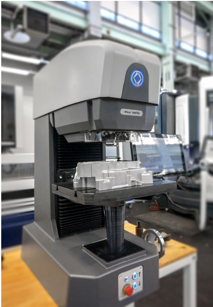
Wilson UH4750 with AlMgSi casting
